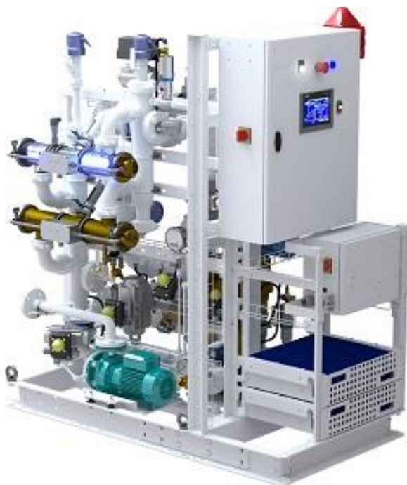
A skid mounted BIO-SEA ballast water treatment system
